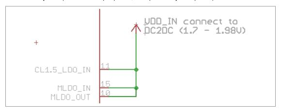
Mixed DC2DC- $V_{BAT}$  system (Maximum RF output power and optimum system power, but requires routing of  $V_{BAT}$ ):
