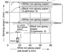
These curves show the characteristics with the maximum sensing range set to 100mm, 200mm, each, with white non-glossy paper  $(50\times50\text{mm})$ .
