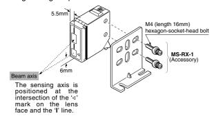
Care must be taken regarding the sensor mounting direction with respect to the object's direction of movement.
